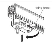
Push the adapter into track till it snaps into place. Turn the mechanical fixing knob. Select the deisired circuit.
