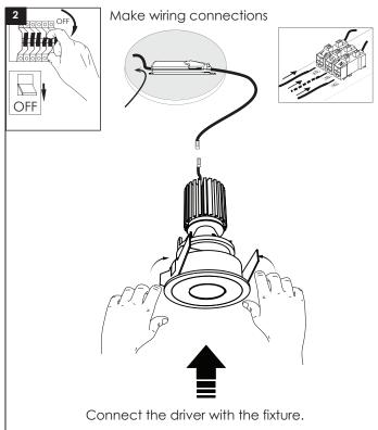
Bend the springs of the fixture and fit it into the false ceiling.
