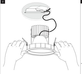
Bend the springs to place the fixture into the ceiling
