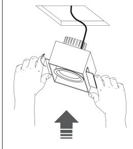
3 Secure using retaining screws. Hold the luminaire while using the drill.
