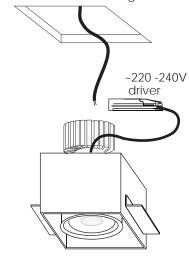
b Make wiring connections
