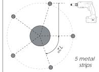
2 Screw on ceiling the metal strips.
