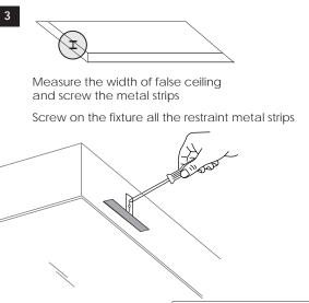
Adjust the position of the strip according to this width
