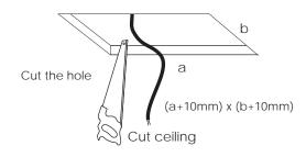
Finish or/and paint the edge of the false ceiling for a better installation result.
