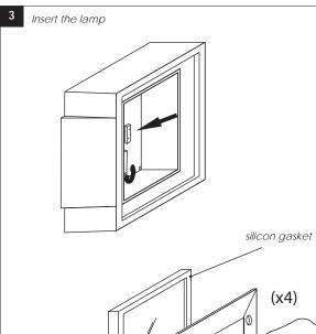
Fit the glass with the silicon gasket on the fixture and then attach the cap.
