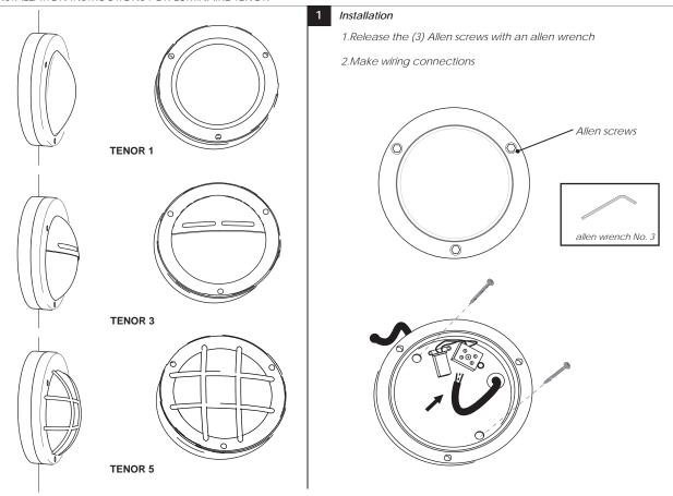
Screw the luminaire on wall or ceiling using screws and wall plugs. Insert the lamp in the lampholder Place the safety glass with the silicone rubber gasket in the fitting and then the cap. Tighten the Allen screws to secure cap.
